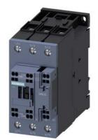
power contactor, AC-3 51 A, 22 kW / 400 V 1 NO + 1 NC, 110 V AC 50 / 60 Hz, 3-pole, size S2, spring-loaded terminal
