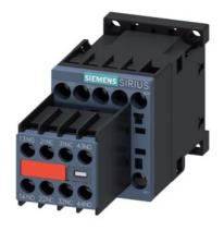
Power contactor, AC-3 9 A, 4 kW / 400 V 2 NO + 2 NC, 24 V DC 3-pole, Size S00 Screw terminal Captive auxiliary switch
