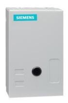
Electrically held lighting contactor, Contactor amp rating 20A, 0 N.C. / 4 N.O. Poles, 24VAC 50/60HZ coil, Non-combination type, (no disconnect device), Enclosure NEMA type 1, Indoor general purpose use
