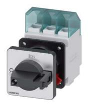
SENTRON, Switch disconnector 3LD, main switch, 3-pole, lu: 25 A, Operating power / at AC-23 A at 400 V: 9.5 kW, front-mounted, knoboperated mechanism, black, central mounting 22.5 mm of the handle
