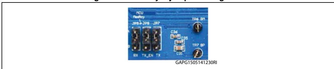
Figure 20. FlexRay – jumper configuration
