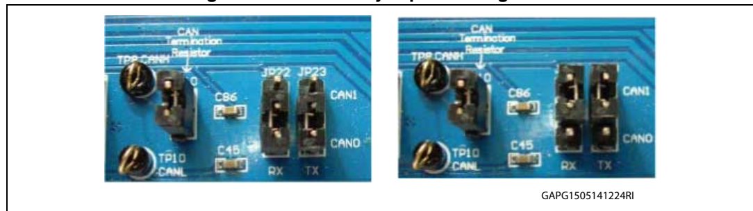
Figure 18. FlexCAN - jumpers configuration
