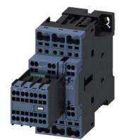
power contactor, AC-3 17 A, 7.5 kW / 400 V 2 NO + 2 NC, 24 V DC, 3-pole, Size S0 Spring-type terminal Removable auxiliary switch
