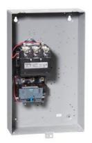
Non-reversing motor starter, Size 3, Three phase full voltage, Solid-state overload relay, OLR amp range 25-100A, 110V 50Hz / 120V 60Hz coil, Non-combination type, Enclosure type 1, Indoor general purpose use, Extra-wide enclosure
