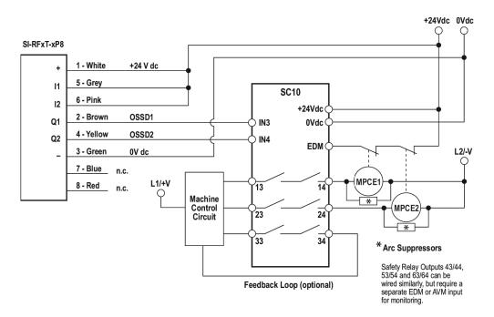
Figure 5: Wiring for a single 8-conductor sensor
