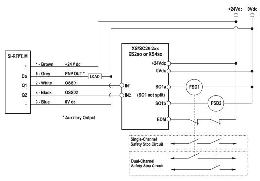
Figure 4: Wiring for a single PNP
