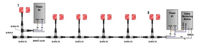
Figure 8: Option 1: Use a SI-RFA-TK Reset Connector in series with ISD Device. If available, set the power supplies for parallel output.
