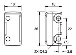
Figure 3: SI-RF Safety Switch -A2 Actuator
