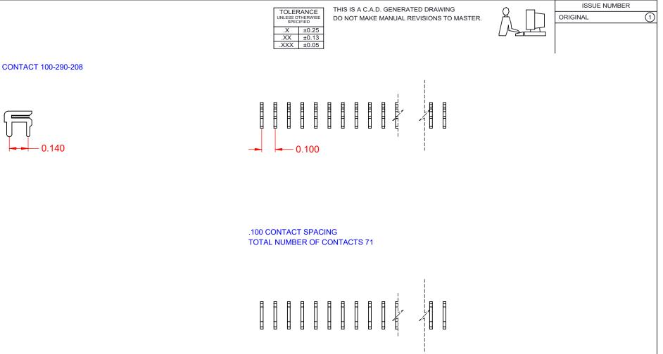
NOTE: CONTACTS ARE HELD IN A CARRIER FOR EASE OF ASSEMBLY
