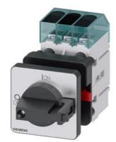
Load disconnector 3LD3, lu 40 A Main switch 3-pole Rated operating capacity at AC-23 A at 400 V 18.5 kW Front plate mounting Basic switch with Central hole mounting 22.5mm Toggle drive black 48x48 mm
