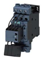
Capacitor contactor, AC-6b 33 kVAr, / 400 V 1 NO + 2 NC, 50-60 Hz AC 95-130 V DC 3-pole, Size S0 screw terminal
