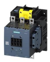
Power contactor, AC-3 150 A, 75 kW / 400 V Coil AC 50/60 Hz and DC 96-127 V x (0.8-1.1) F-PLC input 24 V DC 3-pole size S6 Auxiliary contacts 2 NO + 2 NC Main circuit: Busbar Control and auxiliary circuit: screw terminal
