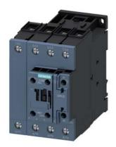
Contactor, AC-1, 60 A/400 V/40 °C, S2, 4-pole, 24 V AC, 50/60 Hz, 1 NO+1 NC, screw terminal
