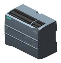
SIPLUS S7-1200 CPU 1215C DC/DC/DC based on 6ES7215-1AG40-0XB0 with conformal coating, -40...+60 °C, start up -25 °C, compact CPU, DC/DC/DC, 2 PROFINET ports, onboard I/O: 14 DI 24 V DC; 10 DQ 24 V DC; 2 AI 0-10 V DC, 2 AQ 0-20 mA DC, power supply: DC 20.4-28.8 V DC, program/data memory 125 KB
