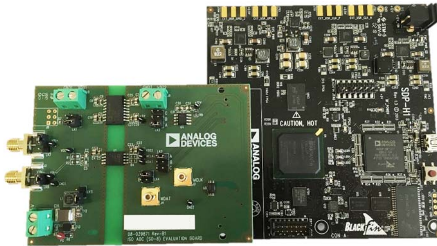
Figure 11. EV-ADuM7701-8FMCZ Evaluation Board (Left) and EVAL-SDP-CH1Z Board (Right) Connection
