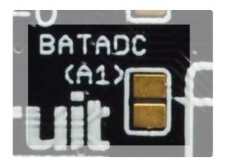
This will allow you to read the voltage level of the LIPO cell using pin A1 where each value on the ADC is equal to 0.80566mV since:
