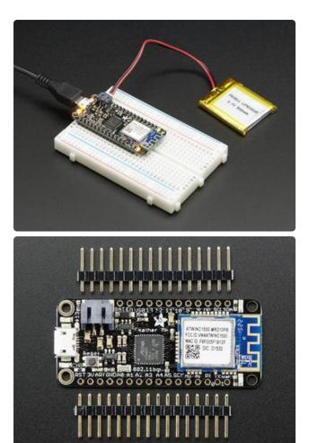
The first option is soldering in plain male headers, this lets you plug in the Feather into a solderless breadboard
