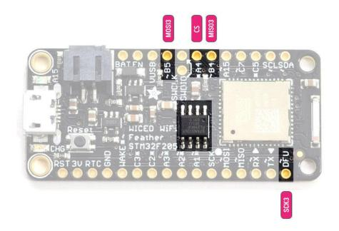
SPI flash is disabled by default. It can be enabled by soldering the SPIFCS (A4) solder jumper on the back of the PCB closed before powering the board up, which will connect the CS/SSEL of the SPI flash to pin A4:
