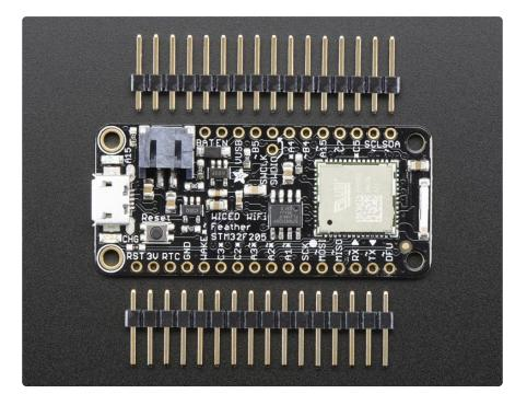
Comes fully assembled and tested, with a USB bootloader that lets you quickly use it with the Arduino IDE. We also toss in some headers so you can solder it in and plug into a solderless breadboard. Lipoly battery () and MicroUSB cable () not included (but we do have lots of options in the shop if you'd like!)
