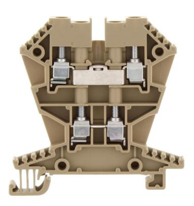
Ex double-level terminal ATEX-certified, Screw connection, Mounting type:Mounting rail TS 35/7.5 and TS 32, Rated cross-section: 4 mm², Width: 6 mm, Colour: Beige
