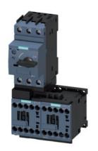
Load feeder fuseless, Reversing duty 400 V AC, Size S00 0.22...0.32 A 24 V DC screw terminal for installation on standard mounting rail (also fulfills type of coordination 1) Type of coordination 2, Iq = 150 kA 1 NC (contactor)
