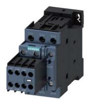
power contactor, AC-3 17 A, 7.5 kW / 400 V 3 NO + 2 NC with 3RH2911-1HA21, 24 V DC, with plugged-in diode combination, 3-pole, Size S0, screw terminal
