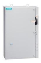
Non-reversing motor starter, Size 0, Three phase full voltage, Solid-state overload relay, OLR amp range 3-12A, 208VAC 60Hz coil, Combination type, 10A circuit breaker, Enclosure NEMA type 4/12, Water/dust tight for outdoors, Extra-wide enclosure
