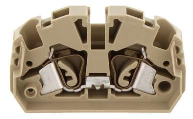
Feed-through terminal for direct mount, Tension-spring connection, Mounting type: Mounting surface, Rated cross-section: 2.5 mm<sup>2</sup>, Width: 11.1 mm, Colour: Beige
