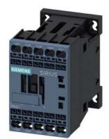
Coupling contactor relay, 2 NC+2 NO 30 V DC, 0.7-1.25\*US with diode integrated Size S00 spring-type terminal suitable for PLC outputs
