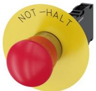
EMERGENCY STOP mushroom-type actuator, 22 mm, round, metal, shiny, red, 40 mm, positive latching, according to EN ISO 13850, rotate-tounlatch, with yellow backing plate, inscription: NOT-HALT, with holder, 1 NO+1 NC, screw terminal, Z=20-unit packaging
