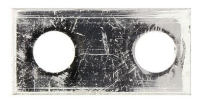
Cross-connector, No. of poles: 2, Mounting type: Can be screwed on, Width: 41 mm, Rated cross-section: 50 mm², Colour: natural
