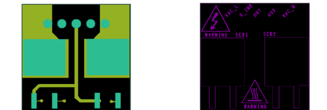
Figure 16. STEVAL-SCR001V1 board layout and silk-screen (bottom side)
