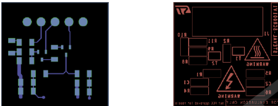
Figure 16. STEVAL-SCR001V1 board layout and silk-screen (bottom side)
