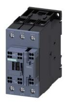
Power contactor, AC-3 80 A, 37 kW / 400 V 1 NO + 1 NC, 230 V AC 50/60 Hz, 3-pole Size S2, Spring-type terminals Upright mounting position
