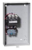
Non-reversing motor starter, Size 3, Three phase full voltage, Solid-state overload relay, OLR amp range 25-100A, Non-combination type, Enclosure type 1, Indoor general purpose use, Standard width enclosure
