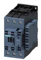
Power contactor, AC-3 65 A, 30 kW / 400 V 2 NO + 2 NC, 230 V AC, 50 Hz 3-pole, size S2 Spring-type terminals lateral auxiliary switch block
