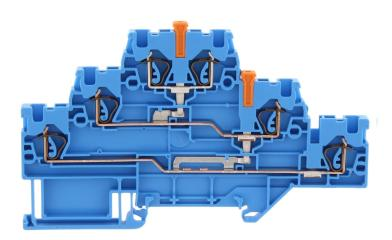
Three-level initiator terminal | Multi-wire terminal, Tension-spring connection, Mounting type: Mounting rail TS 35/7.5, Rated cross-section: 2.5 mm², Width: 5.1 mm, Colour: Blue
