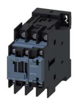
contactor relay, AC-3 32 A, 15 kW / 400 V 1 NO + 1 NC, 24 V DC with integrated varistor 3-pole, size S0 ring cable lug connection suitable for PLC outputs not expandable with auxiliary switch
