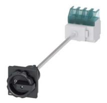
SENTRON, Switch disconnector 3LD, main switch, 4-pole, lu: 25 A, Operating power / at AC-23 A at 400 V: 9.5 kW, floor mounting with door coupling, rotary operating mechanism, black, 4-hole mounting of the handle
