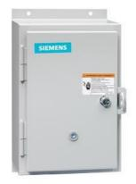
Non-reversing motor starter, Size 1, Three phase full voltage, Solid-state overload relay, OLR amp range 3-12A, Non-combination type, Enclosure type 12, Dust/drip proof for indoors, Extra-wide enclosure
