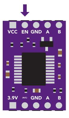
Setting the EN pin to low will shut off the Basic EZO<sup>™</sup> Inline Voltage Isolator, along with the connected circuit. The current consumption will be reduced to **3.8 mA**.
