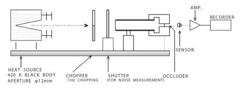
Figure 2 - Occluder Position
