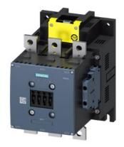
Contactor, AC-1, 400 A/690 V/40 °C, S10, 3-pole, 200-277 V AC/DC, F-PLC-IN with varistor, 2 NO+2 NC, Connection rail/ screw terminal
