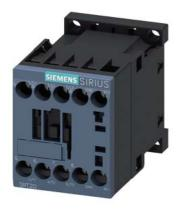
power contactor, AC-3 12 A, 5.5 kW / 400 V 1 NC, 24 V DC 0.7-1.25\*US 3-pole, size S00 screw terminal suitable for PLC outputs not expandable with auxiliary switch
