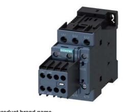
power contactor, AC-3 25 A, 11 kW / 400 V 2 NO + 2 NC, 125 V DC, 3-pole, Size S0 screw terminal Removable auxiliary switch
