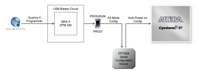
Figure 3-5 The AS Configuration Scheme
