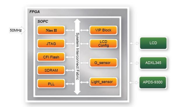
Figure 4-16 Block diagram of the digital accelerometer demonstration
