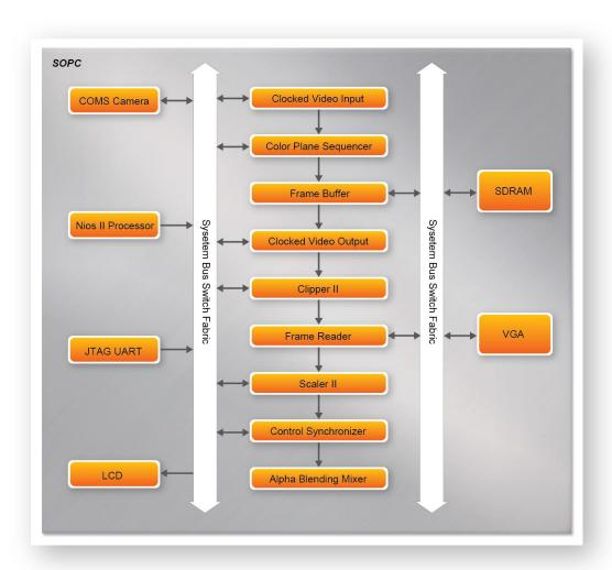
Figure 4-14 VIP Camera Example SOPC Block Diagram (Key Components)
