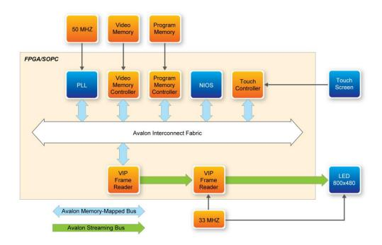
Figure 4-2 Block diagram of the Painter demonstration
