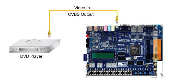
Figure 4-11 Setup for the VIP demonstration
