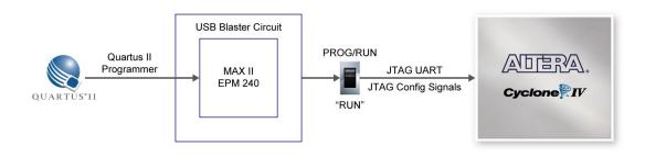
Figure 3-3 JTAG Chain Configuration Scheme
