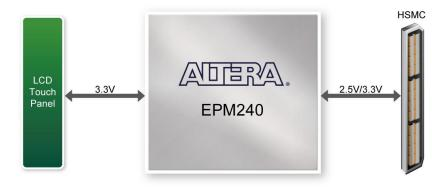
Figure 3-6 Block Diagram of the Bus Controller
