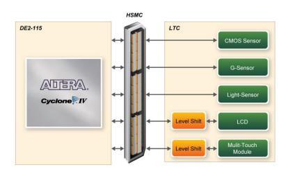
Figure 2-3 Block Diagram of VEEK-MT
