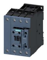
Power contactor, AC-3 40 A, 18.5 kW / 400 V 2 NO + 2 NC 20-33 V AC/DC 4-pole size S2 screw terminals 1 NO + 1 NC integrated
