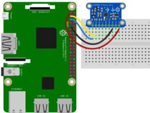
Pi 3V3 to sensor Vin Pi GND to sensor GND Pi SCL to sensor SCL
