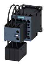
Capacitor contactor, AC-6b 12.5 kVAr, / 400 V 1 NO + 1 NC, 24 V AC, 50/60 Hz 3-pole, Size S00 screw terminal
