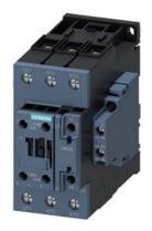
Power contactor, AC-3 65 A, 30 kW / 400 V 2 NO + 2 NC, AC / DC 20-33 V, with varistor 3-pole, size S2 screw terminals lateral auxiliary switch block
