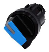
Selector switch, illuminable, 22 mm, round, plastic, blue, selector switch, short, 2 switch positions O-I, latching, actuating angle  $90^\circ$ , 10:30h/13:30h
