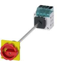
Load disconnector 3LD3, lu 63 A Main switch 3-pole + N Rated operating capacity at AC-23 A at 400V 22.0 kW floor mounting Basic switch with door coupling Central hole mounting 22.5mm Rotary actuator red / yellow 66 x 66 mm with auxiliary switch 10E + 1S
