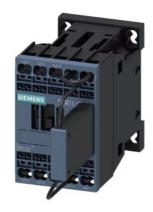
Traction contactor, AC-3 9 A, 4 kW / 400 V 72 V DC 0.7-1.25\* US, with varistor integrated, 3-pole, Size S00, Spring-type terminal
