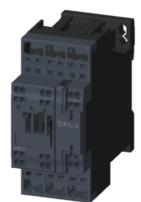
Power contactor, AC-3 32 A, 15 kW / 400 V 1 NO + 1 NC, 230 V AC 50/60 Hz, 3-pole Size S0, Spring-type terminals
