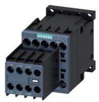
Power contactor, AC-3 9 A, 4 kW / 400 V 2 NO + 2 NC, 24 V DC 3-pole, Size S00 screw terminal Removable auxiliary switch
