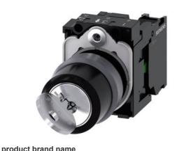
RONIS key-operated switch, 22 mm, round, plastic with metal front ring, lock number SB30, with 2 keys, 2 switch positions O-I, latching, actuating angle 90°, 10:30h/13:30h, key removal O+I, with holder, 1 NO, screw terminal, possible special locks: SB31, 421, 455, with laser labeling, upper case and lower case, always upper case at the beginning of the word
