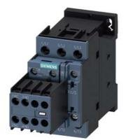
power contactor, AC-3 9 A, 4 kW / 400 V 2 NO + 2 NC, 24 V AC, 50 Hz 3-pole, Size S0 screw terminal Removable auxiliary switch
