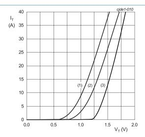
$V_o$  = 1.041 V;  $R_s$  = 0.0179 Ω (1)  $T_j$  = 150 °C; typical values (2)  $T_j$  = 150 °C; maximum values (3)  $T_j$  = 25 °C; maximum values
